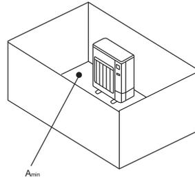
B) Install in a space with a depression height of  $\leq 0.1$  [m].
