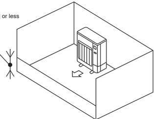
C) Create an opening in the closed face in front of the unit to enable ventilation in the area, ensuring to follow all professional safety instructions and equipment requirements when making the opening through drilling or otherwise.
