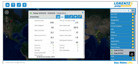
Figure 58: pumpMANAGER view of system details
